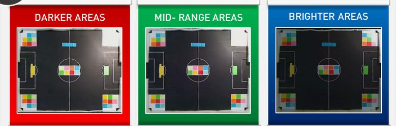
Each camera is adjusted to match a different lighting aspect of the training scene. This ensures all colour patches can be sampled.
