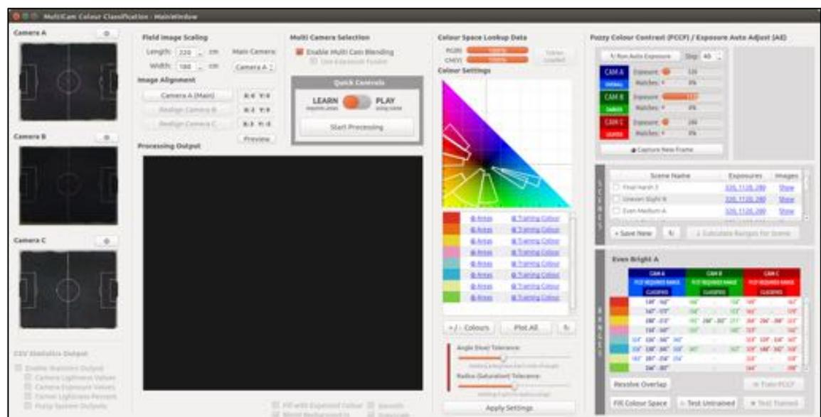
This program facilitates the image pre-processing by manually selected homographic points, scales image based on the real-life measurements entered, then automatically aligns each camera. The exposure selection process is run using the defined colours and areas, before allowing lighting scenarios to be saved to file.
