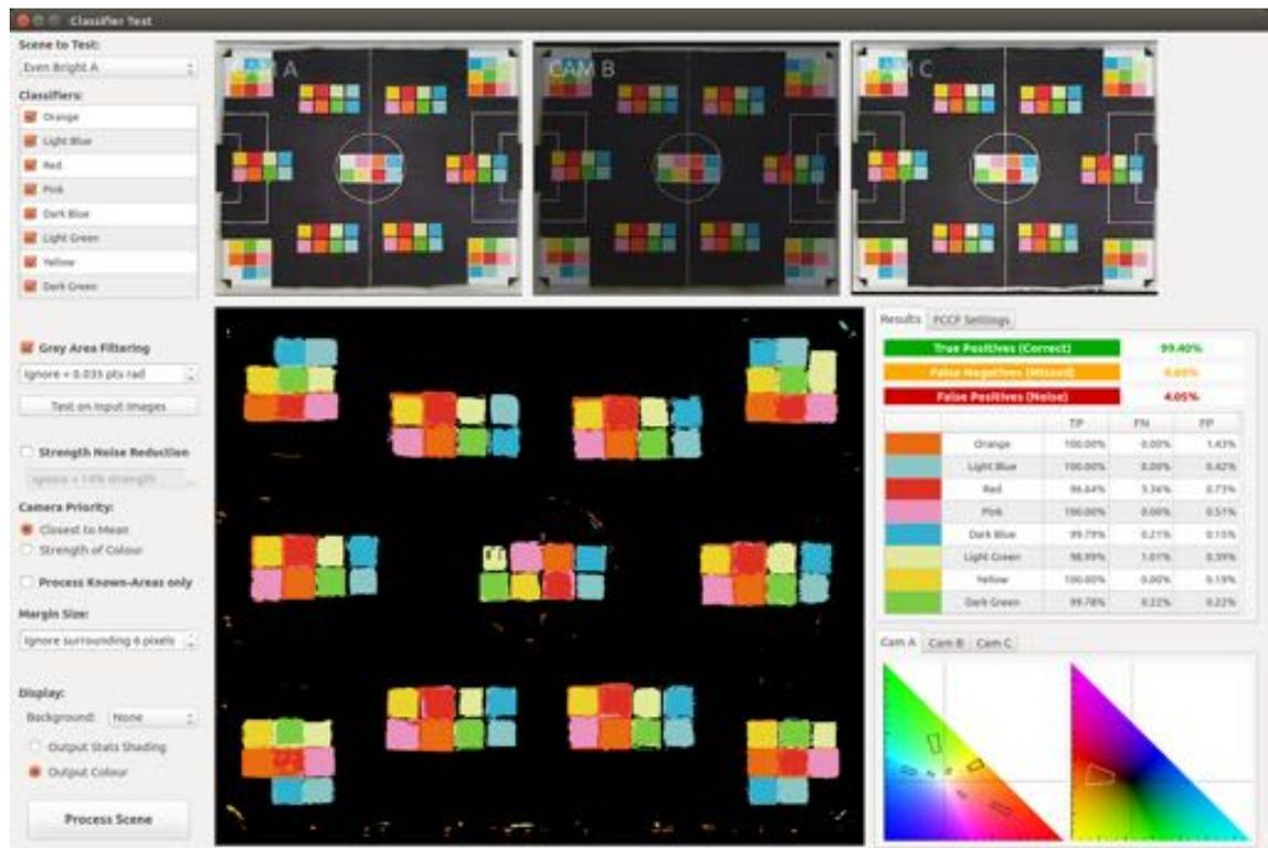
This final program loads each classifier from file, along with a particular lighting scenario. Outputs such as confusion matrices, true positives and false positives are generated here for each scene, saved directly to CSV file for further analysis.
