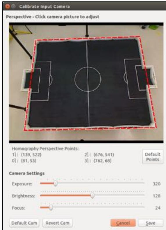
Camera C, shown above, ready for alignment. The homographic points, generated by clicking on the live image, are shown as a red dotted rectangle.
