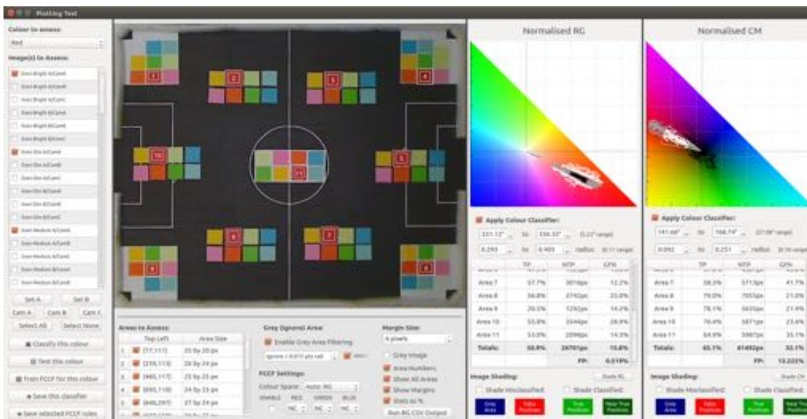
The next program loads the PNG image files and known-areas, plotting data to the two colour spaces. Testing then prioritises one over the other, before saving the classifier to file. As mentioned in Section 4.5, 24 classifiers are saved in total.
